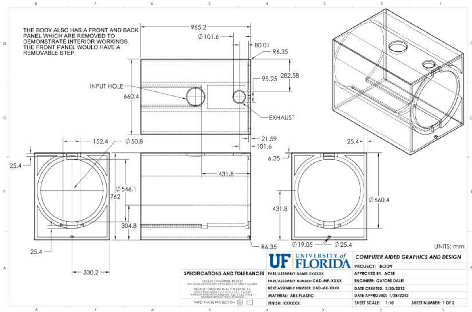
**Drawing 2. Detailed view of subcomponents of the body including labels for major structures.**
