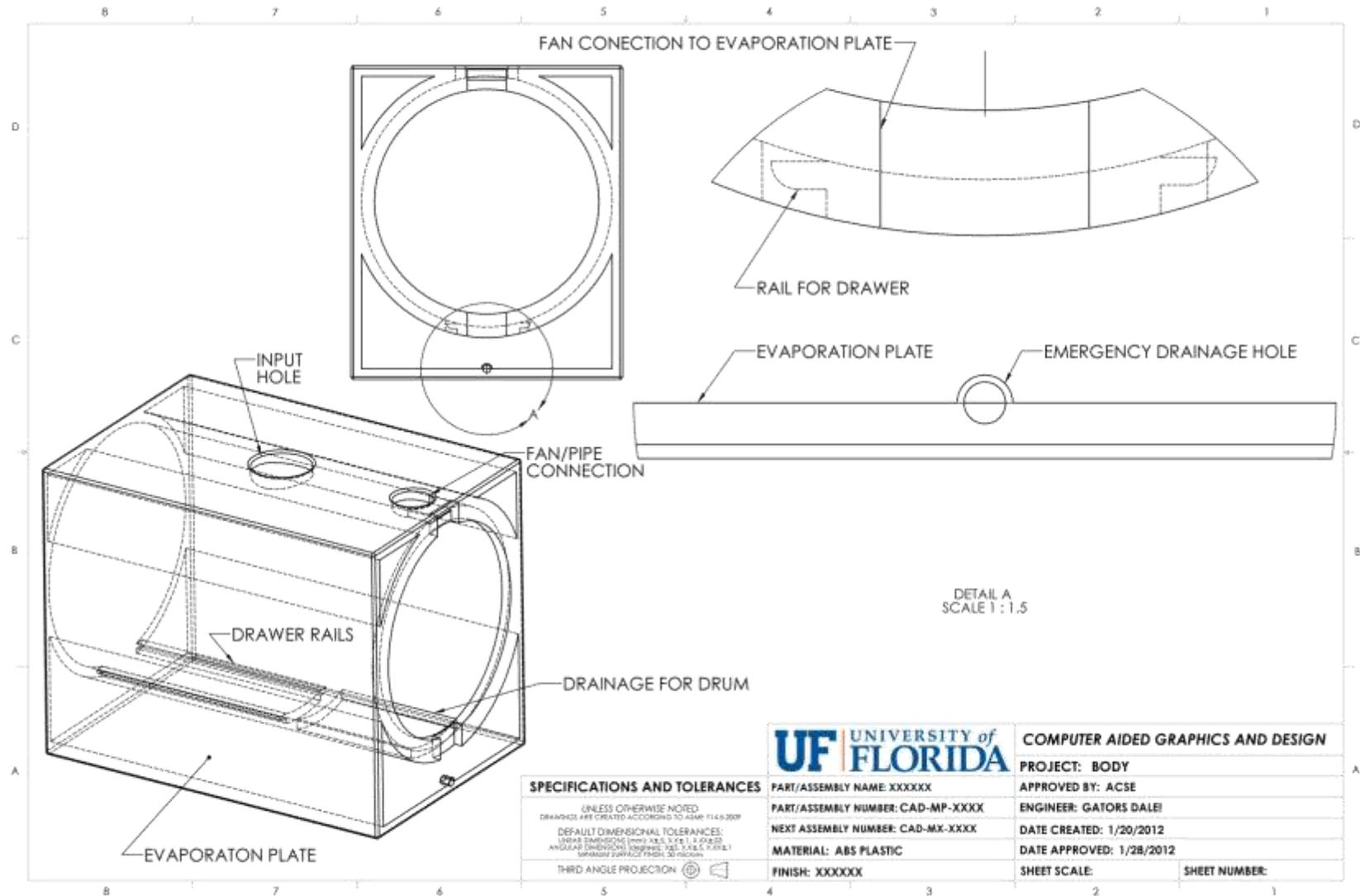
**Drawing 3. Drum along with its design components. The drum is the main compartment in which decomposition of fecal matter occurs. It has an input and output hole along with an array of small holes for the purpose of draining excess moisture due mostly to urine.**
