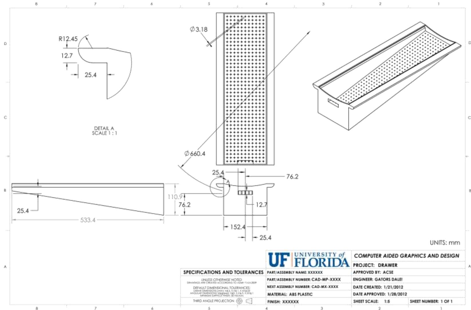
**Drawing 7. Assembly of compost toilet components. Bright colors were used for distinction of components, although the general material of choice is ABS plastic. Front and back panels along with a step and toilet lid have been removed for simplicity.**
