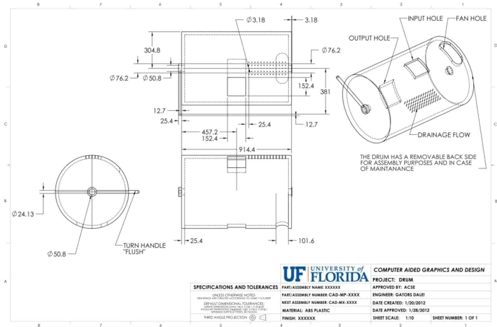
**Drawing 4. Mixer depiction.** It was designed to aerate the fecal matter to provide enough oxygen for complete aerobic decomposition.
